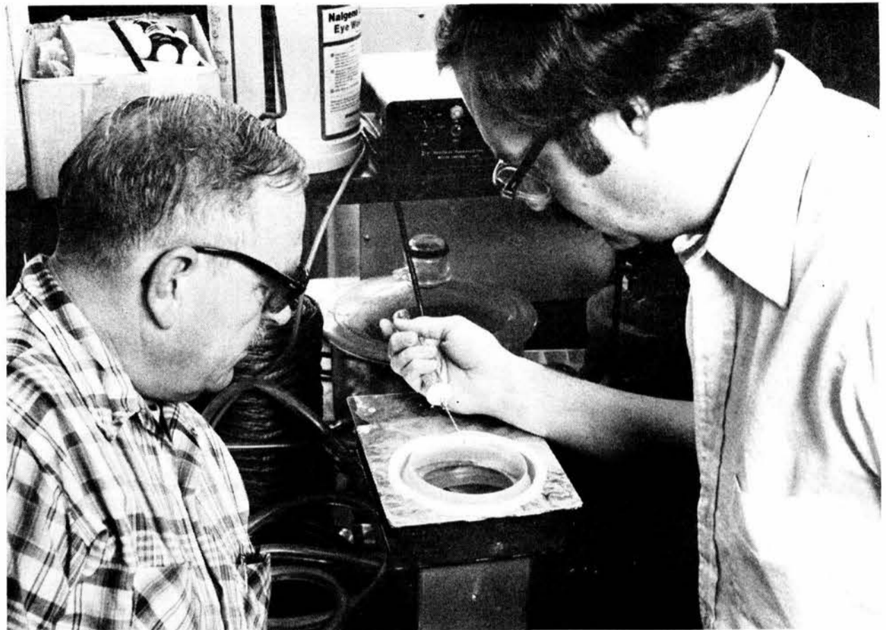
POLYSILANE PHOTORESIST is injected into spin caster via syringe by John Zeigler (1811) as co-developer Larry Harrah (1812) looks on. New silicon-based photoresist is self developing and may lead to significant improvements in the fabrication of microcircuits. (Spin caster is typical method of depositing a photoresist on a silicon wafer.)
